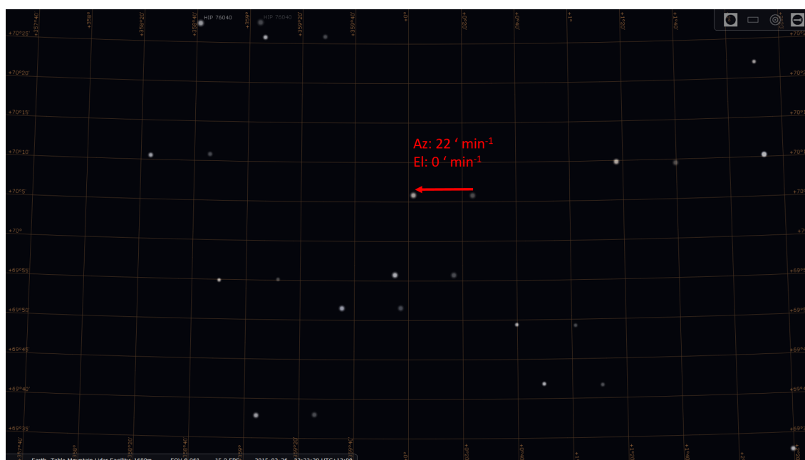
Figure B.7: Drift of star field predicted by Stellarium over sixty seconds while observing northward beam.
